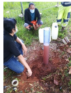
Gambar 2. Pengukuran Falling Head Test .
