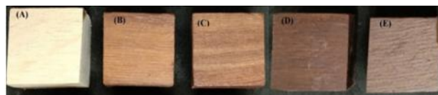
Figure 1. Color changes of Simalambuo wood from the control (A) to treatments at 130 °C (B), 150 °C (C), 170 °C (D), and 190 °C (E).
