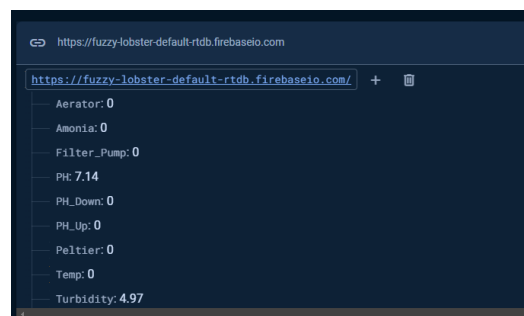
Figure 7. Data is received by the Firebase database in real-time.
