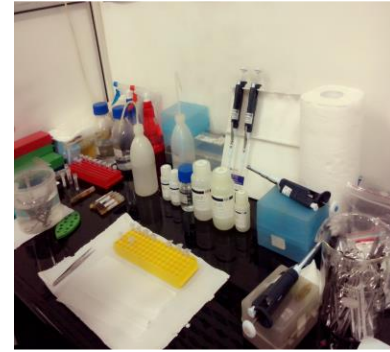
Gambar 1. Persiapan alat dan bahan ekstraksi DNA (gunting, pinset, scalpel, waterbath, sentrifuge, microwave, tabung ependorf 1.5 ml, tip, mikro pipet ukuran 0.1 il - 1000 il, Proteinase K, EtOH absolut).
