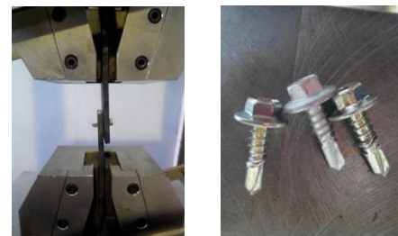
Gambar 9. Pengujian Geser Self Drilling Screw
