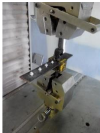
Gambar 10 Pengujian tarik self drilling screw
